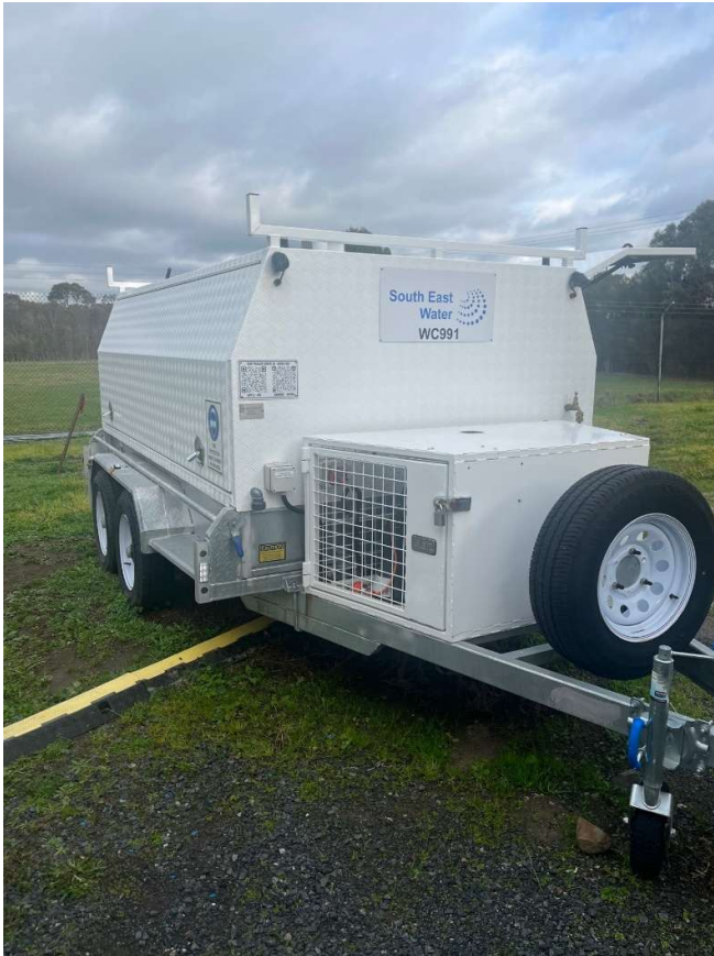
Figure 8 – Emergency mains backup supply system located (on-board) on trailer in secure lockup.
