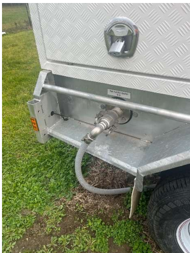
Figure 1 - PDU example of ported connection allowing doors to remain closed and locked when system is operational
