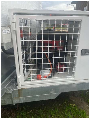
Figure 2 – Example of PDU Generator housing located on A-Frame of trailer
